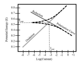
FIGURE C-4. Polarization curve with an Evans Diagram.
