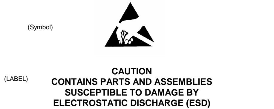
FIGURE 17. Electrostatic discharge (ESD) sensitive identification.
