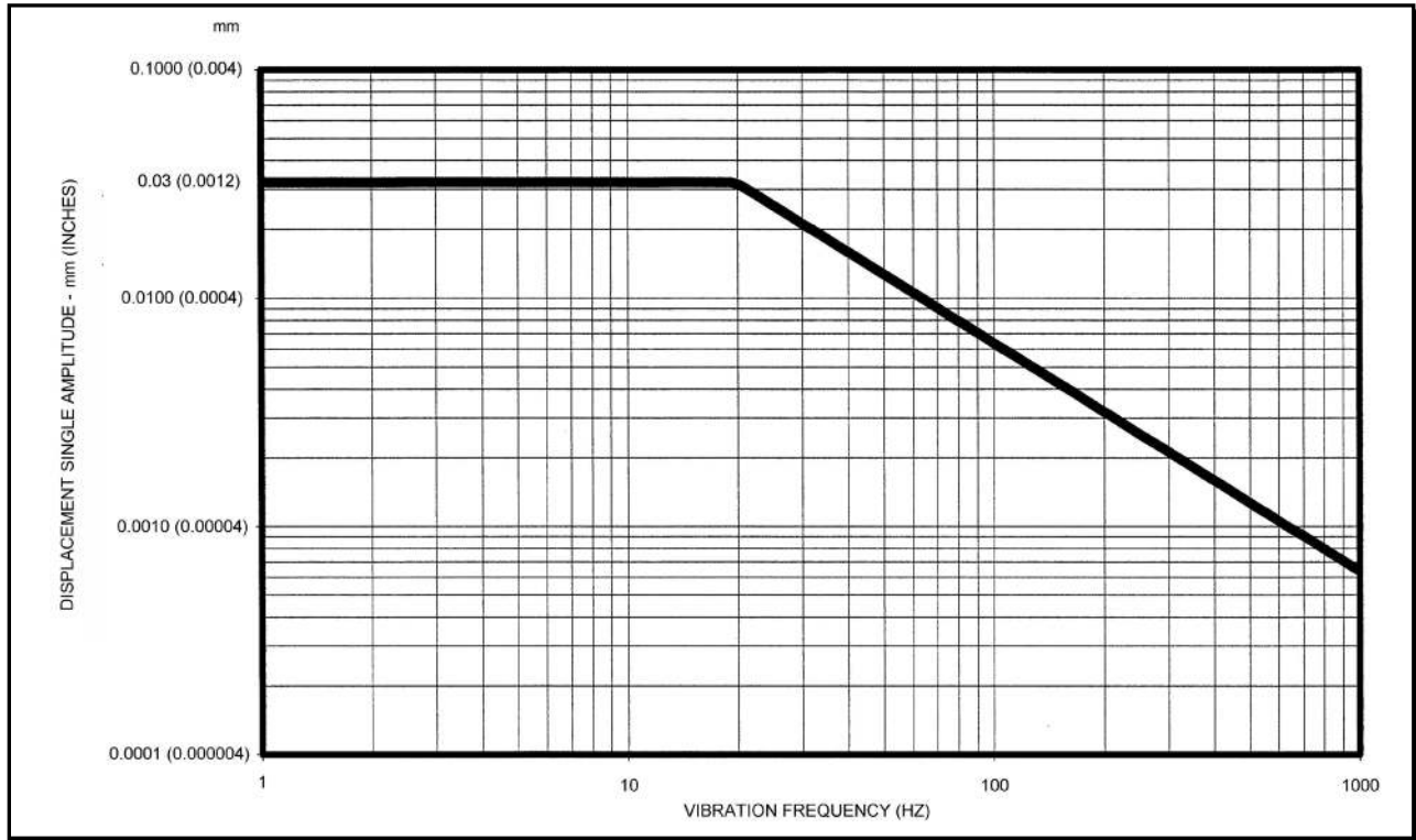
Figure 528.1-2. Vibration acceptance criteria for Type II vibration.
