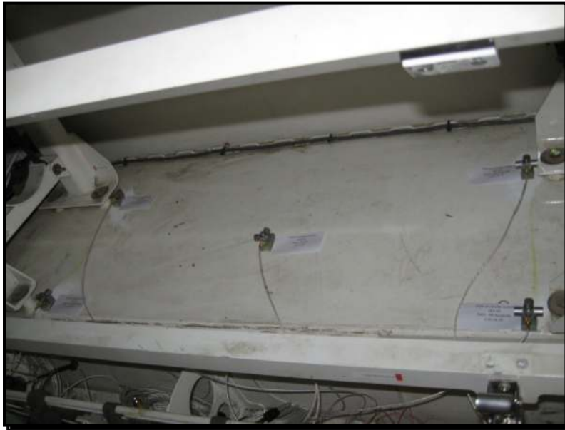
Figure 4. Transducer placement (input to missile rack).
