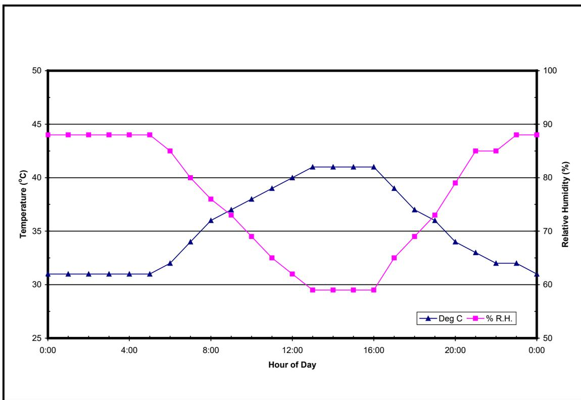
Figure 507.6-6. Natural Cycle B3 - Hot humid.
