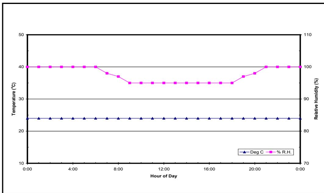
Figure 507.6-4. Natural Cycle B1 – Constant high humidity.
