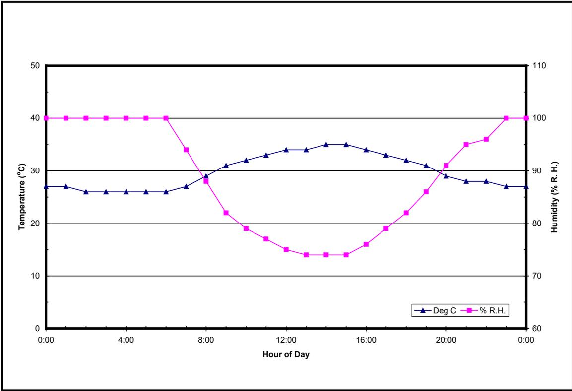
Figure 507.6-5. Natural Cycle B2 – Cyclic high humidity.
