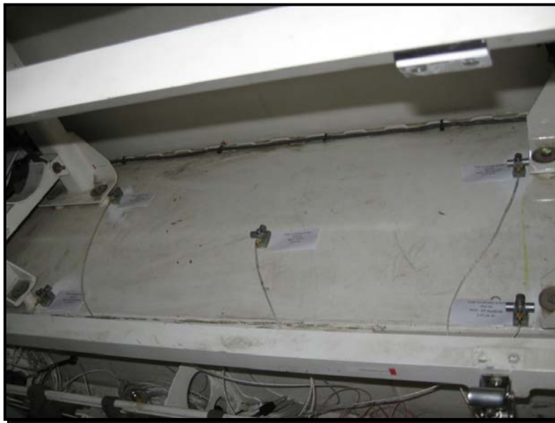
Figure 4. Transducer placement (input to missile rack).
