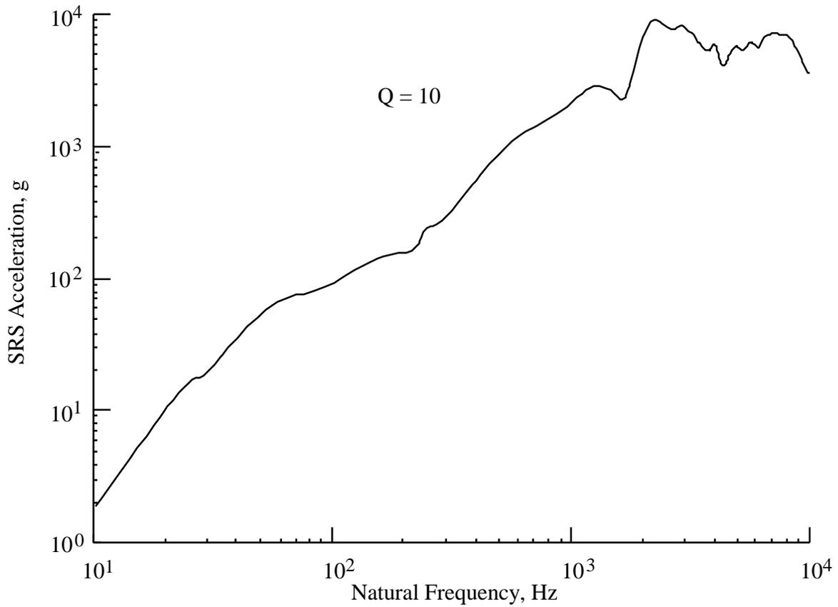
FIGURE 2. Typical Pyroshock Maximax Shock Response Spectrum (SRS)
