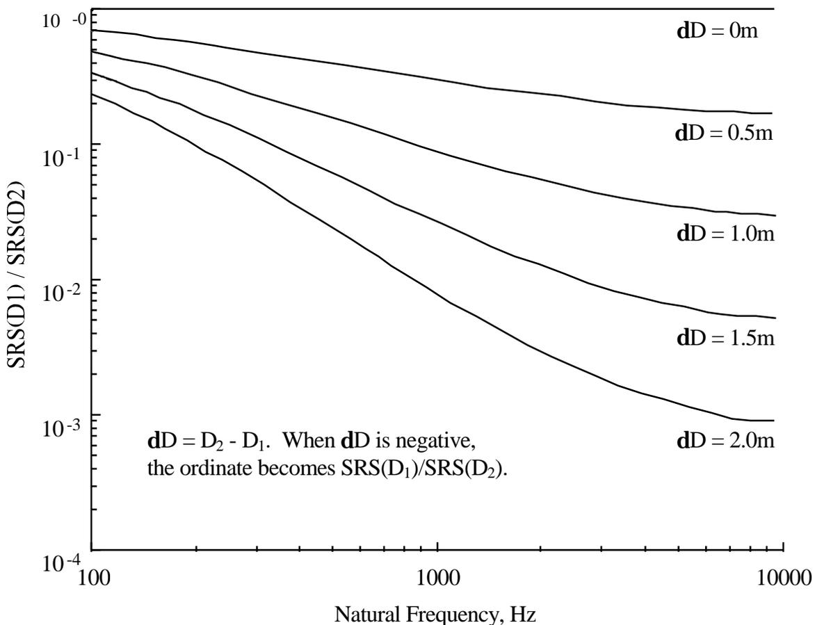
FIGURE A-2. Correction of Shock Response Spectrum for Distance from Pyrotechnic Source
