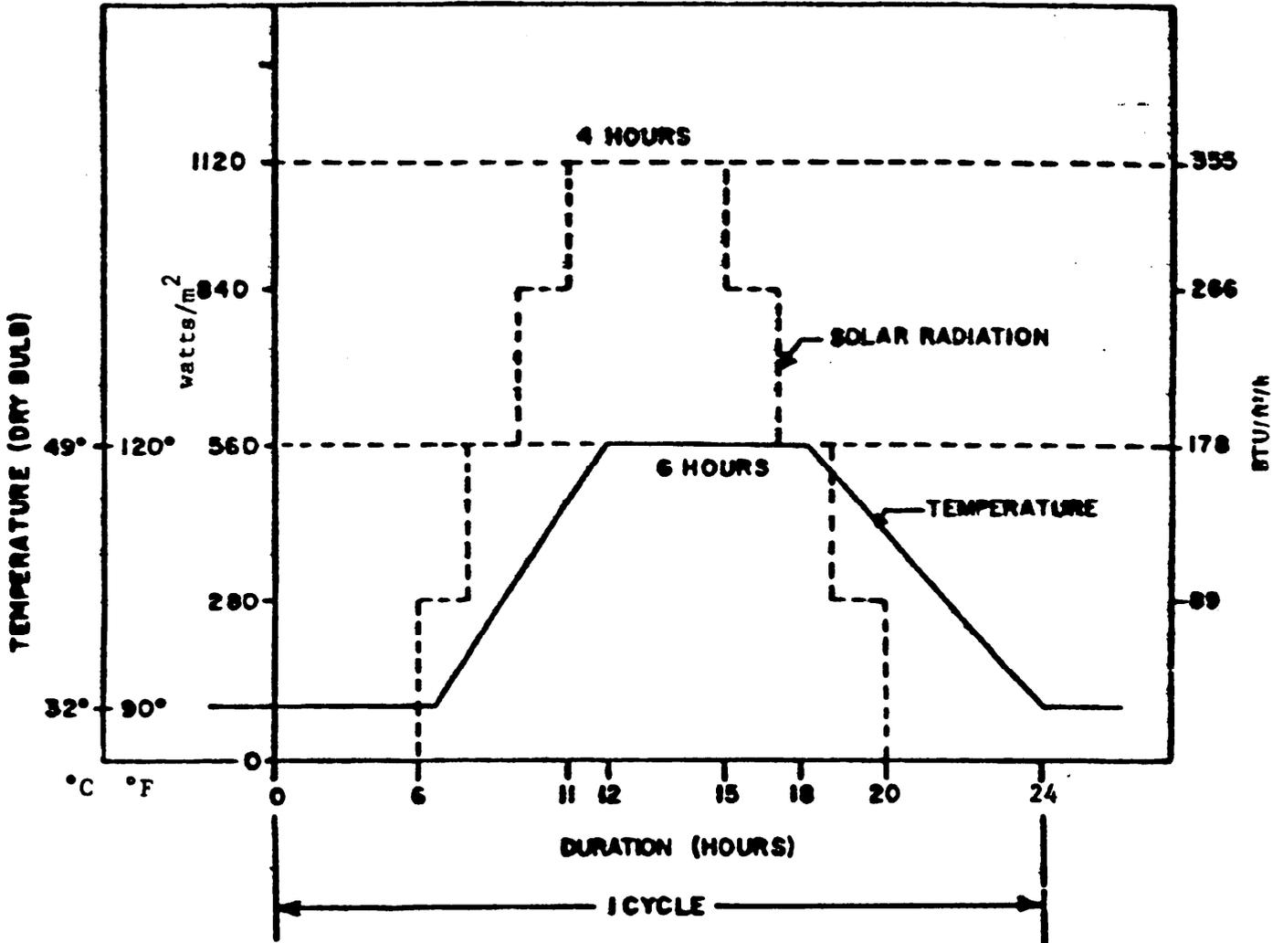
FIGURE 505.3-1 Simulated solar radiation cycle (Procedure I).
