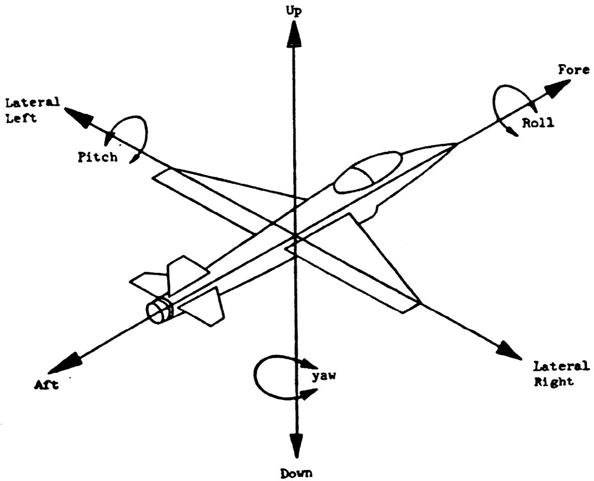
FIGURE 513.4-1. Directions of vehicle acceleration.
