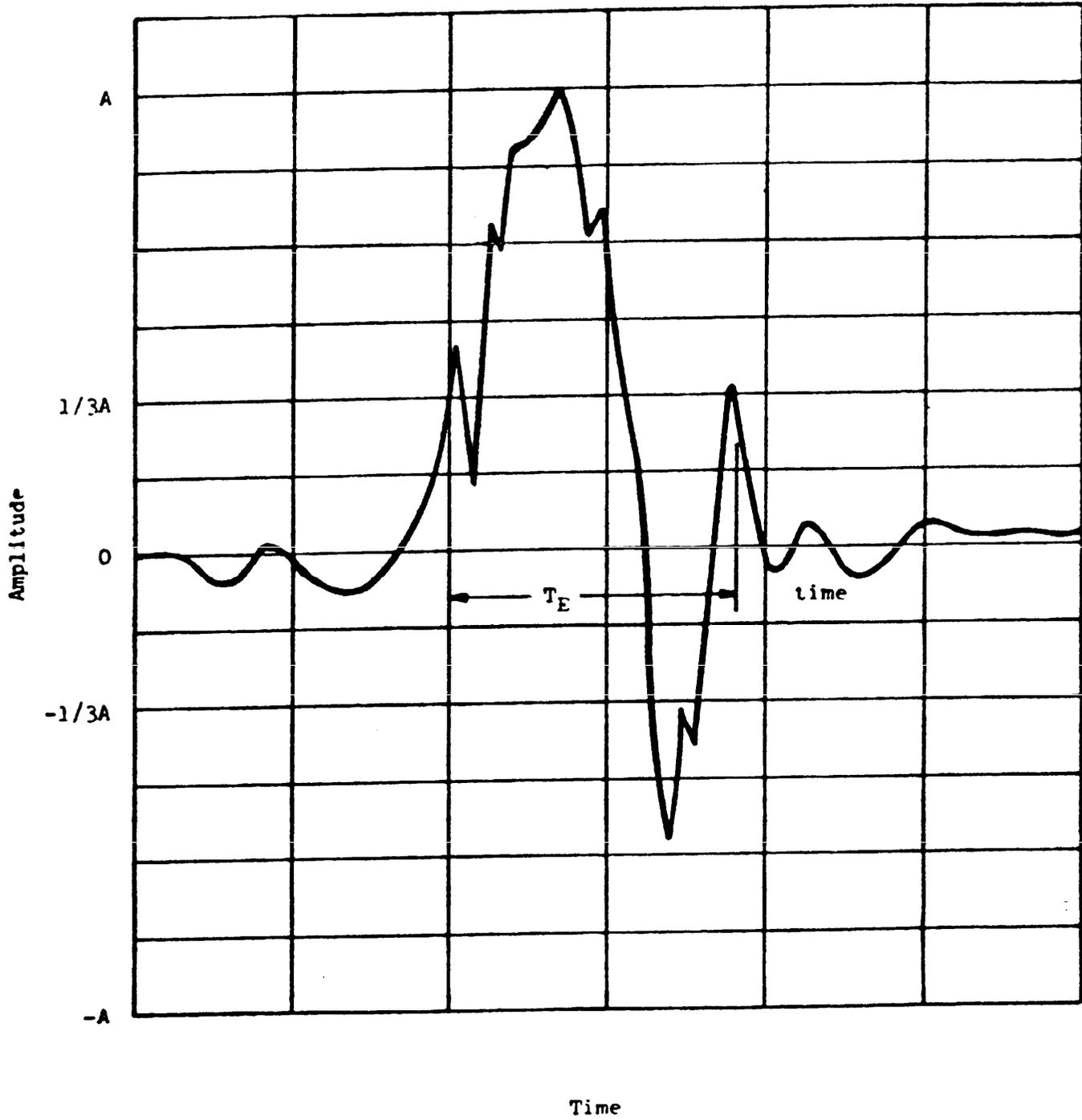
FIGURE 516.4-3. Example of a shock time history showing effective transient duration ( $T_E$ ).
