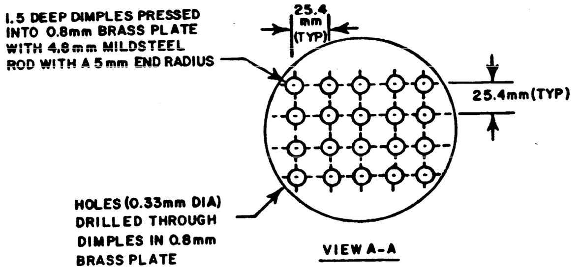
Figure 506.3-1. Details of Dispenser for Drip Test
