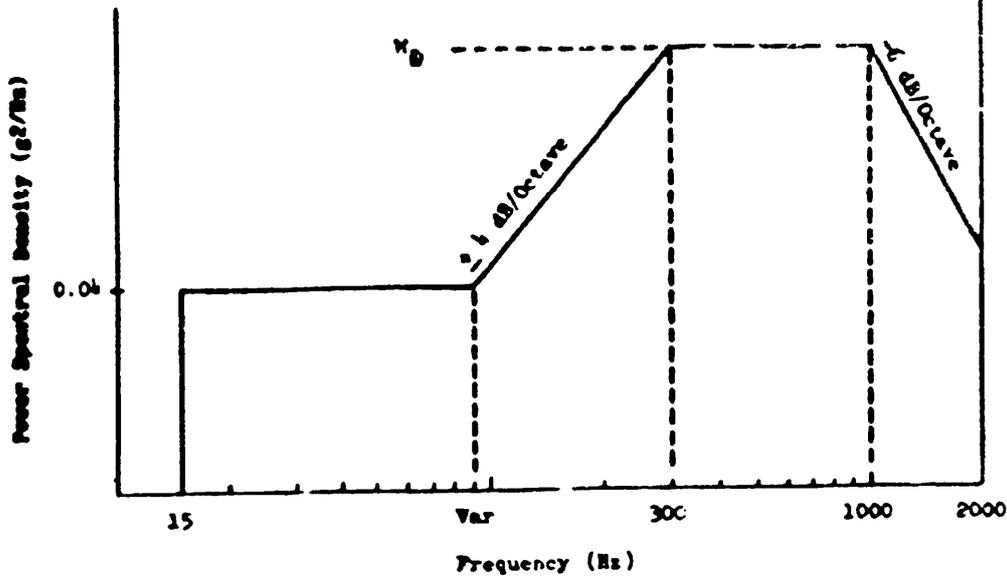
Figure 514.4-8. Suggested vibration levels for high performance aircraft.
