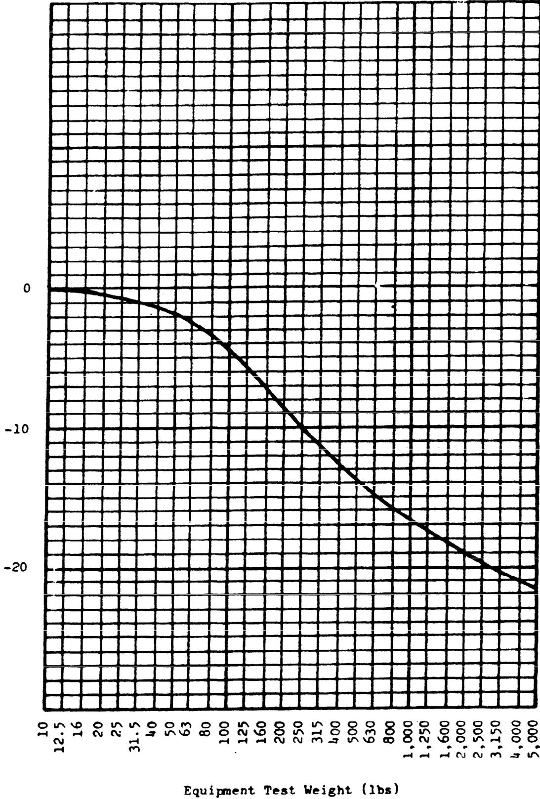
FIGURE 519.45. Test level reduction due to equipment mass loading.
