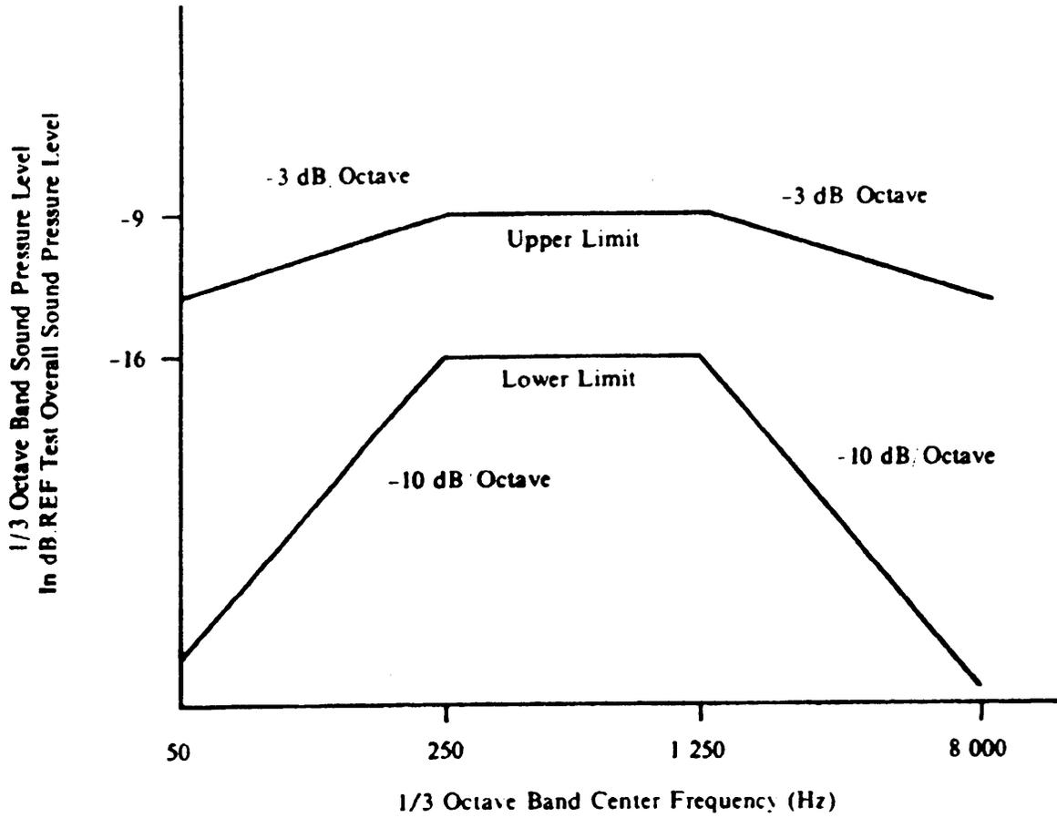
FIGURE 515.4-1. Suggested 1/3 octave band spectra for acoustical noise test.
