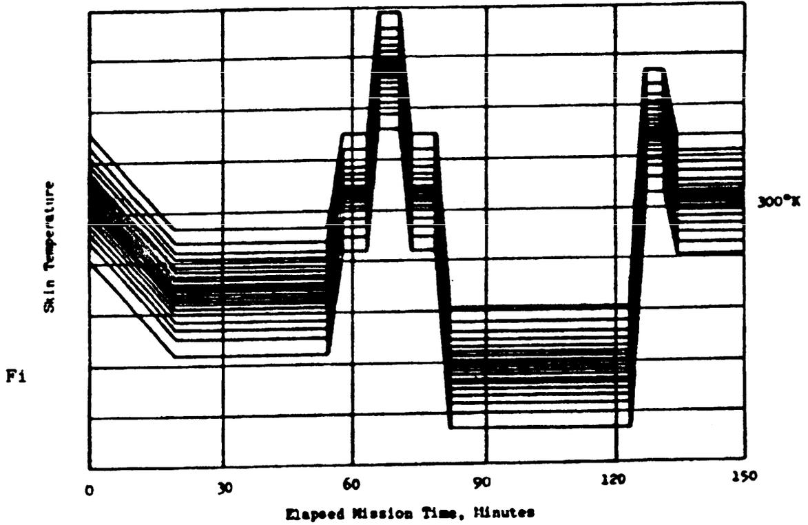
FIGURE 523.1-4. Climatic set of temperature profiles for composite mission.
