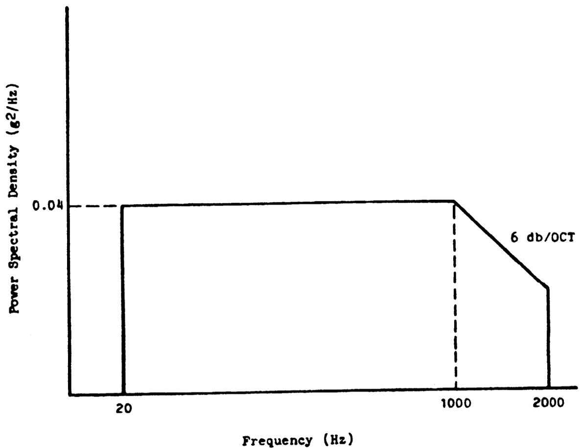
FIGURE 514.4-16 Minimum integrity test-general.
