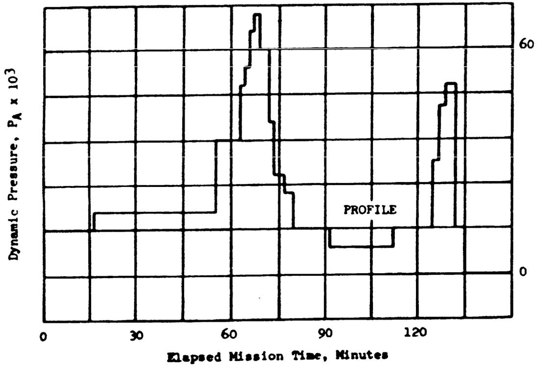
FIGURE 523.1-6 Dynamic pressure, q, profile for composite mission.
