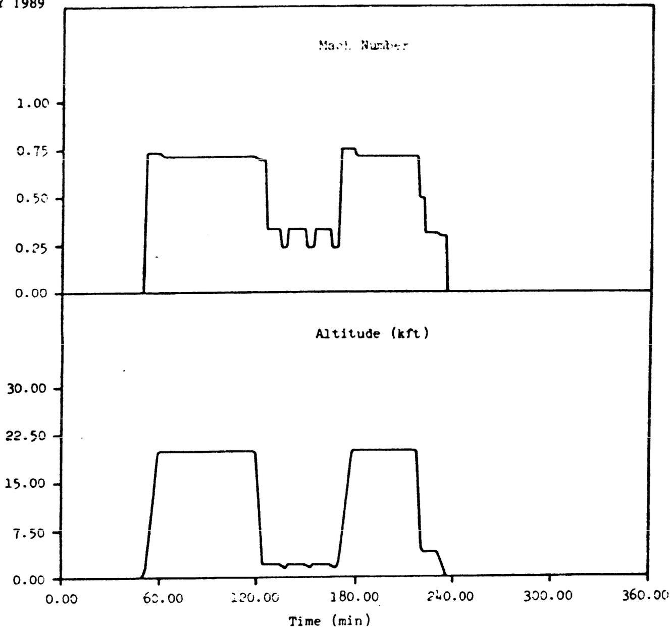
FIGURE 520.1-3. Schematic mission profile, altitude and mach number.
