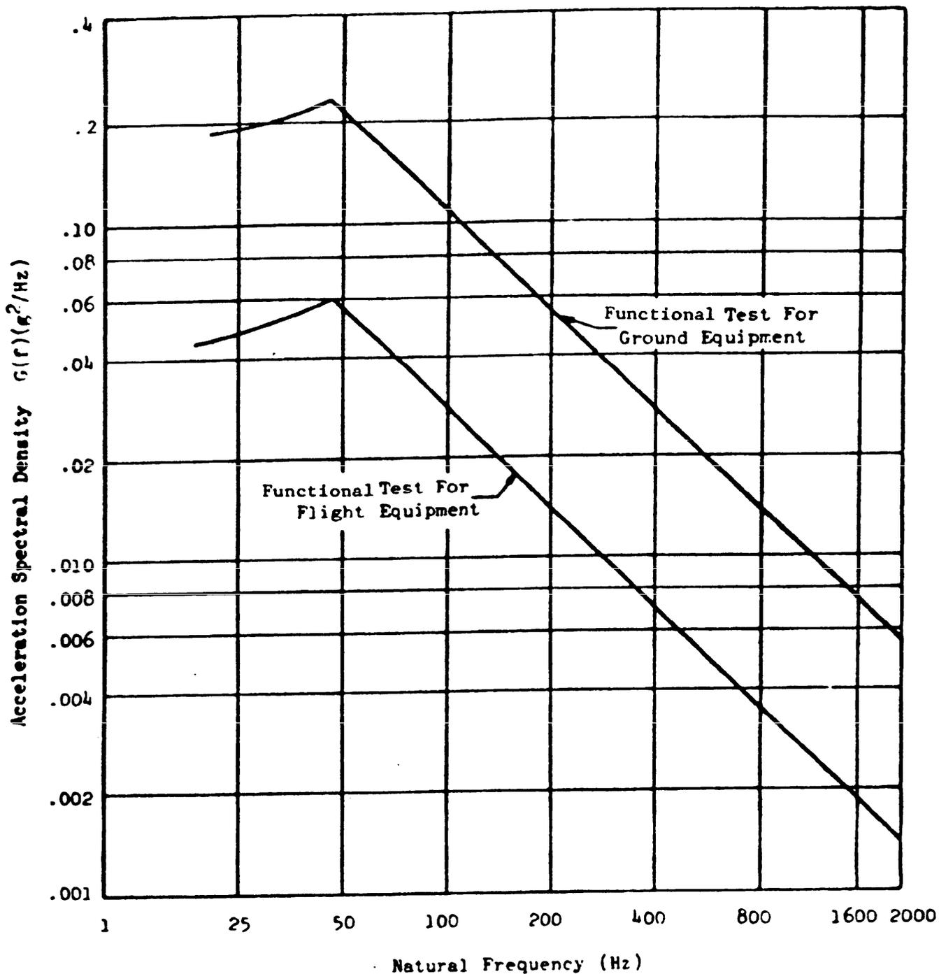
FIGURE 516.4-2. Random test input spectral density yielding equivalent test shock response spectra shown in figure 516.4-1- 516.4-5
