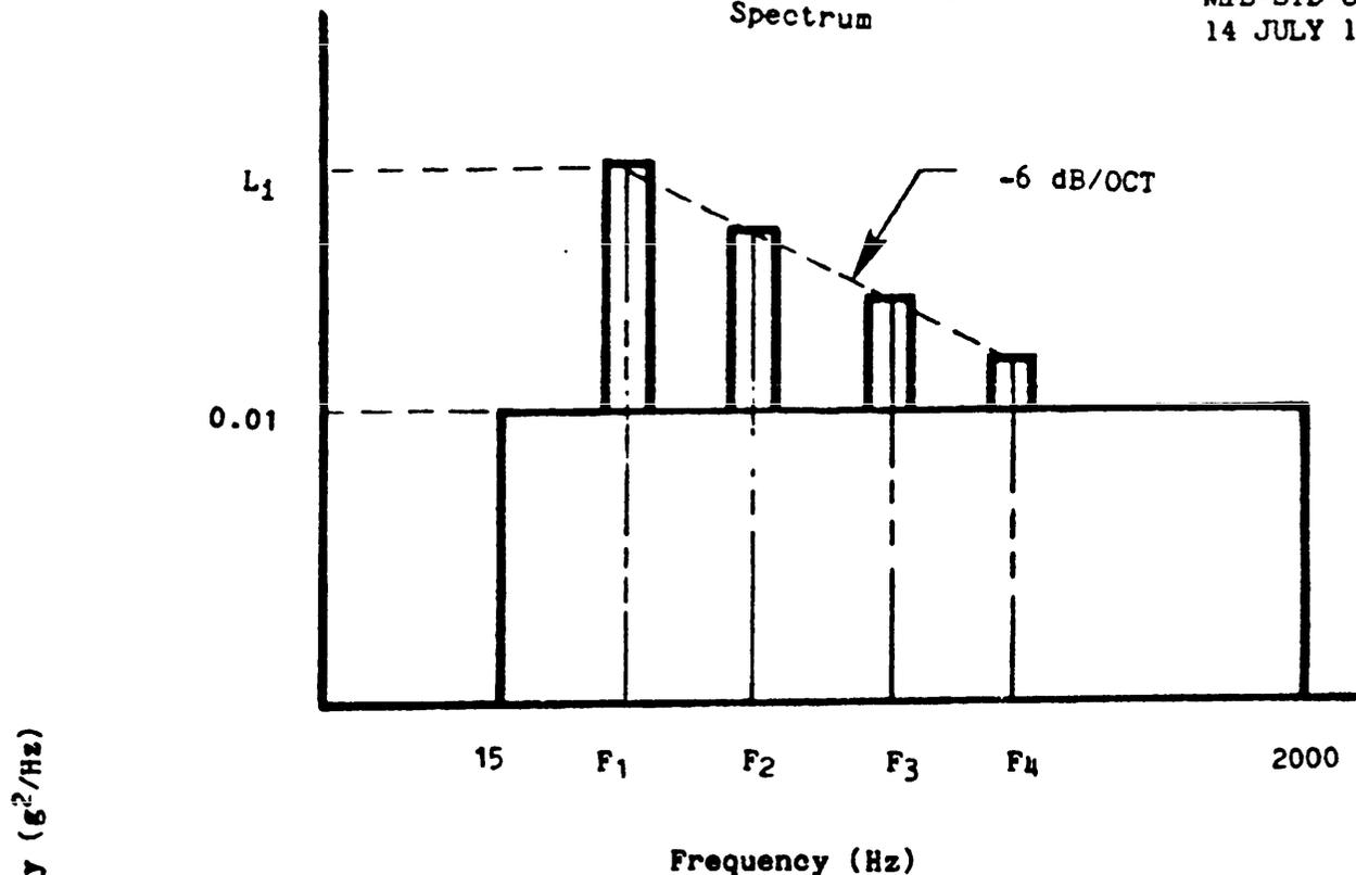
b. Turbine engine spectrum
