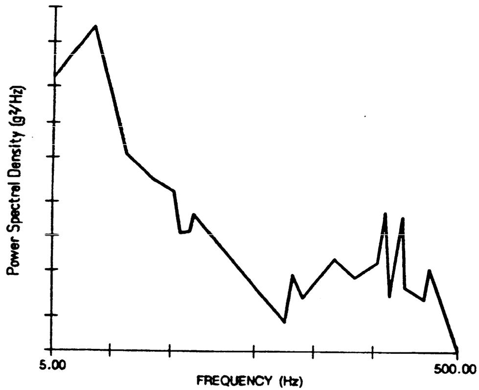
FIGURE 514.4-4 Representative spectral shape, wheeled vehicle.
