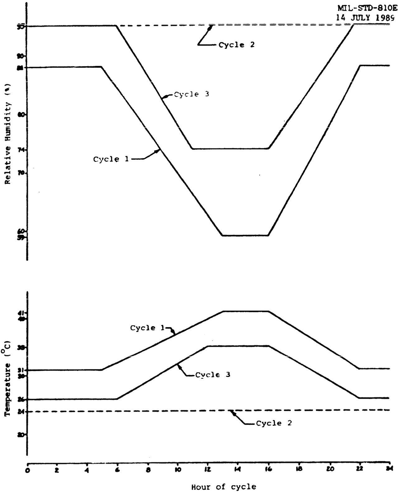
FIGURE 507.3.1. Natural temperature-humidity cycles.
