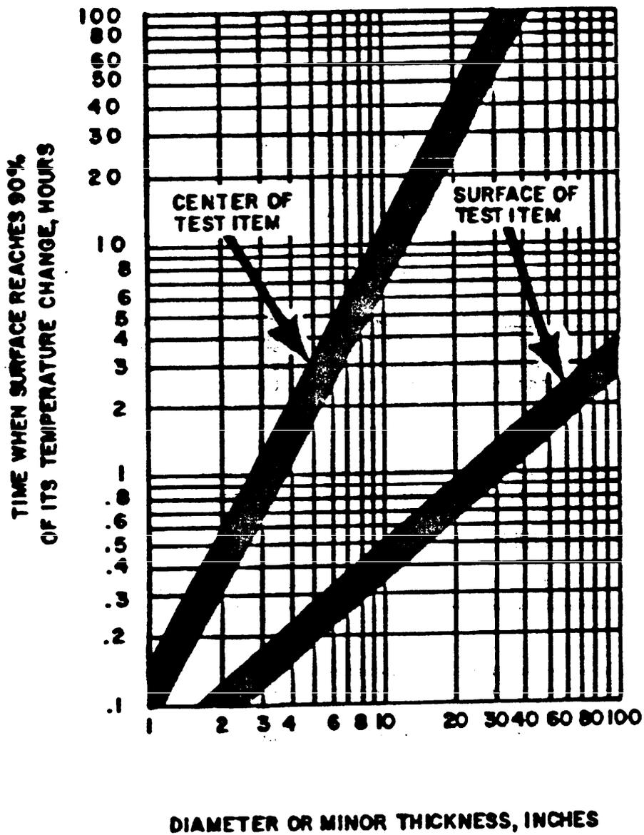
FIGURE 501.3-1 Temperature stabilization curves.
