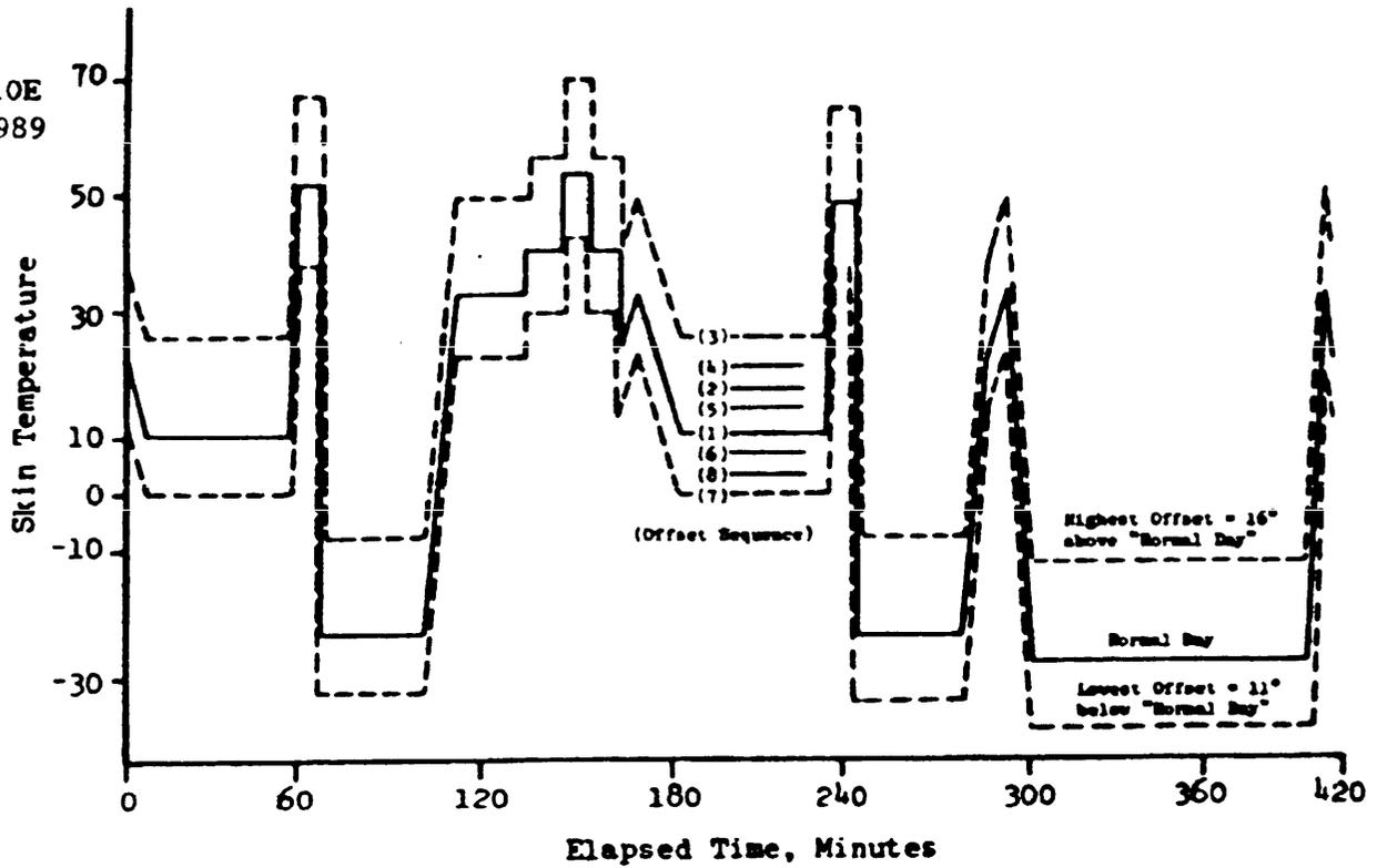
FIGURE 523.1-5 Climatic set plan showing offset sequence.
