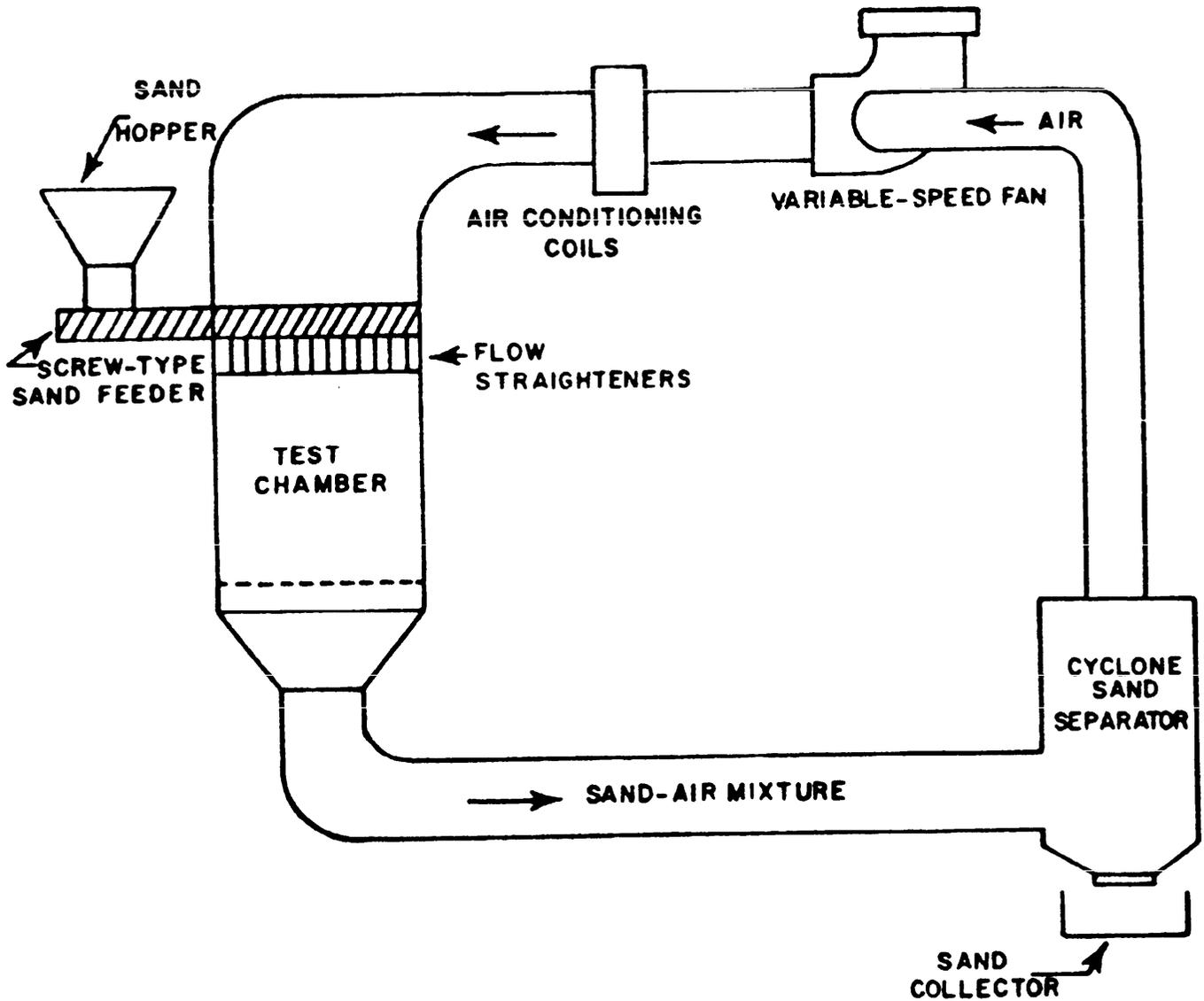
FIGURE 510.3-1. Blowing sand test facility (vertical flow).
