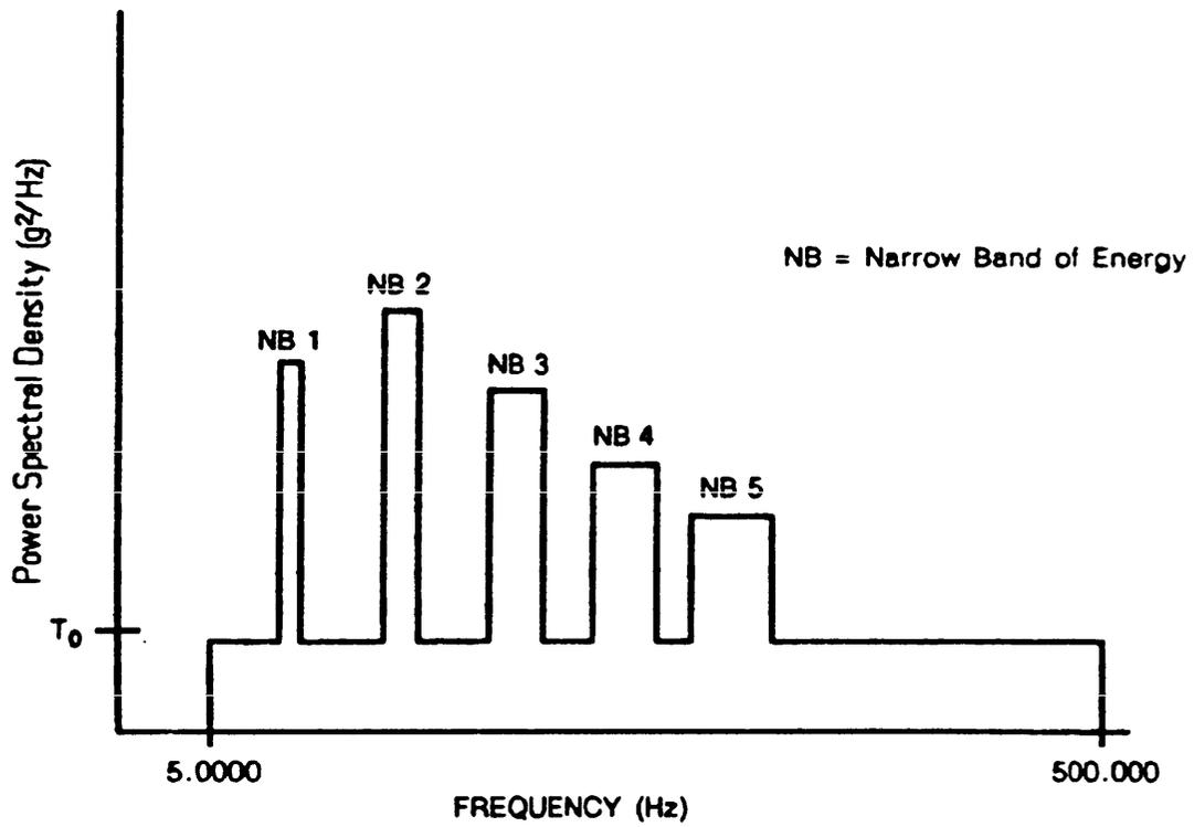
FIGURE 514.4-5. Representative spectral shape, tracked vehicle.
