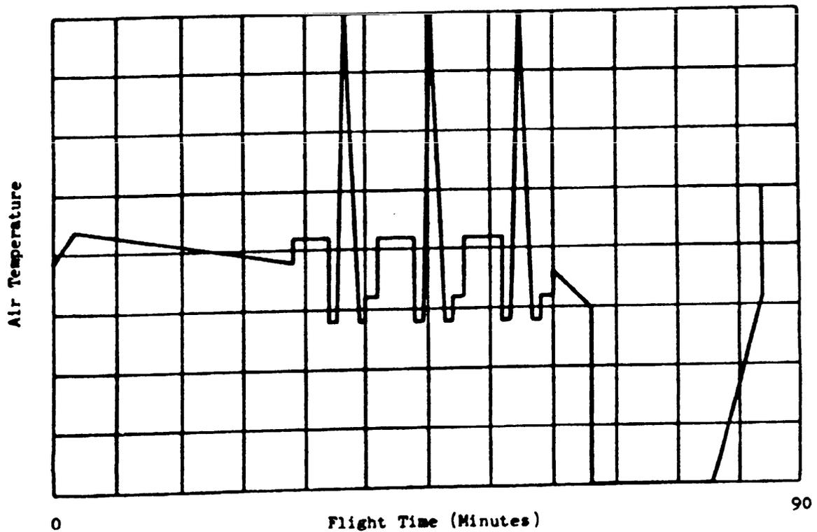
FIGURE 523.1-2. Temperature profile for a single mission type.
