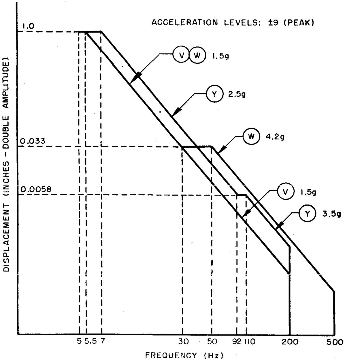
Note: All curves shall be extended to 2 Hz when test item resonances below 5 Hz are expected
