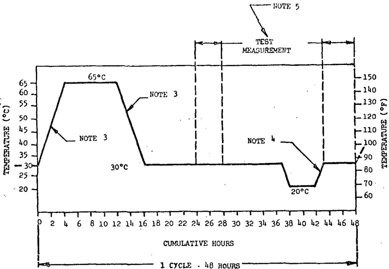
FIGURE 507.1-2. Humidity Cycle Procedures II and III
