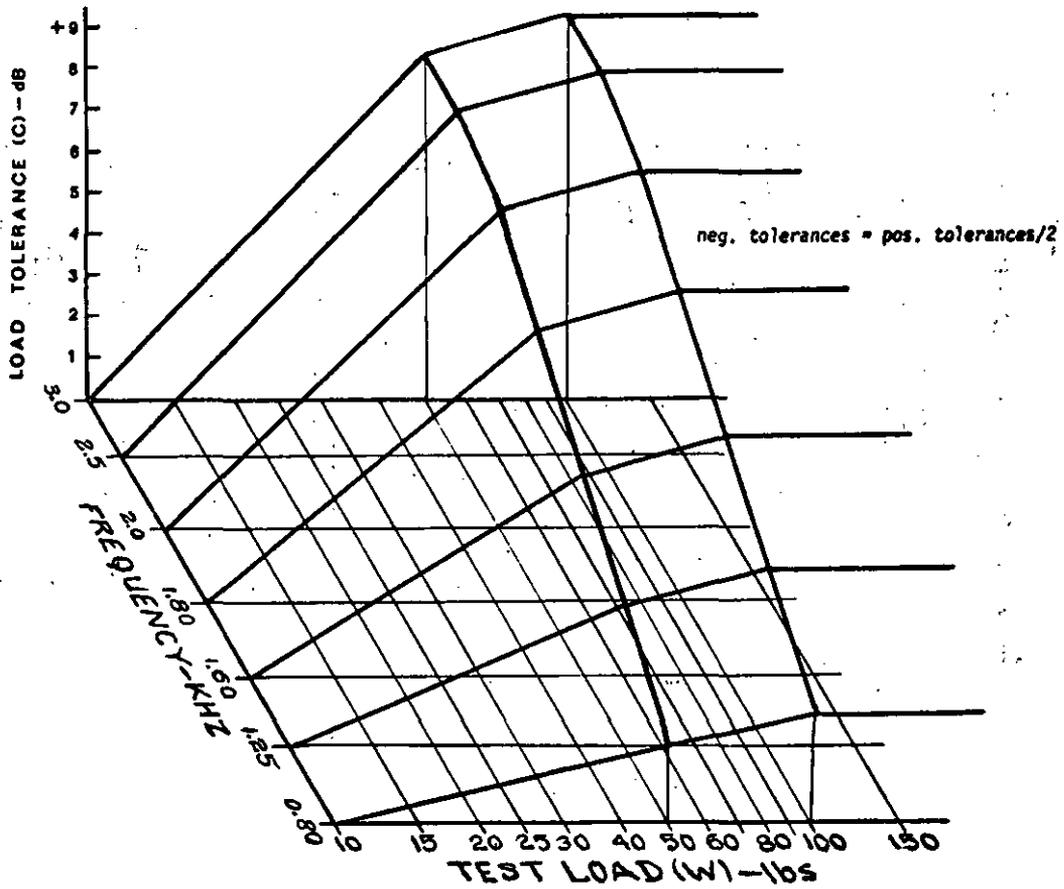
FIGURE 519.2-22 Gunfire test tolerance (C) for W ≥ 10 lbs
