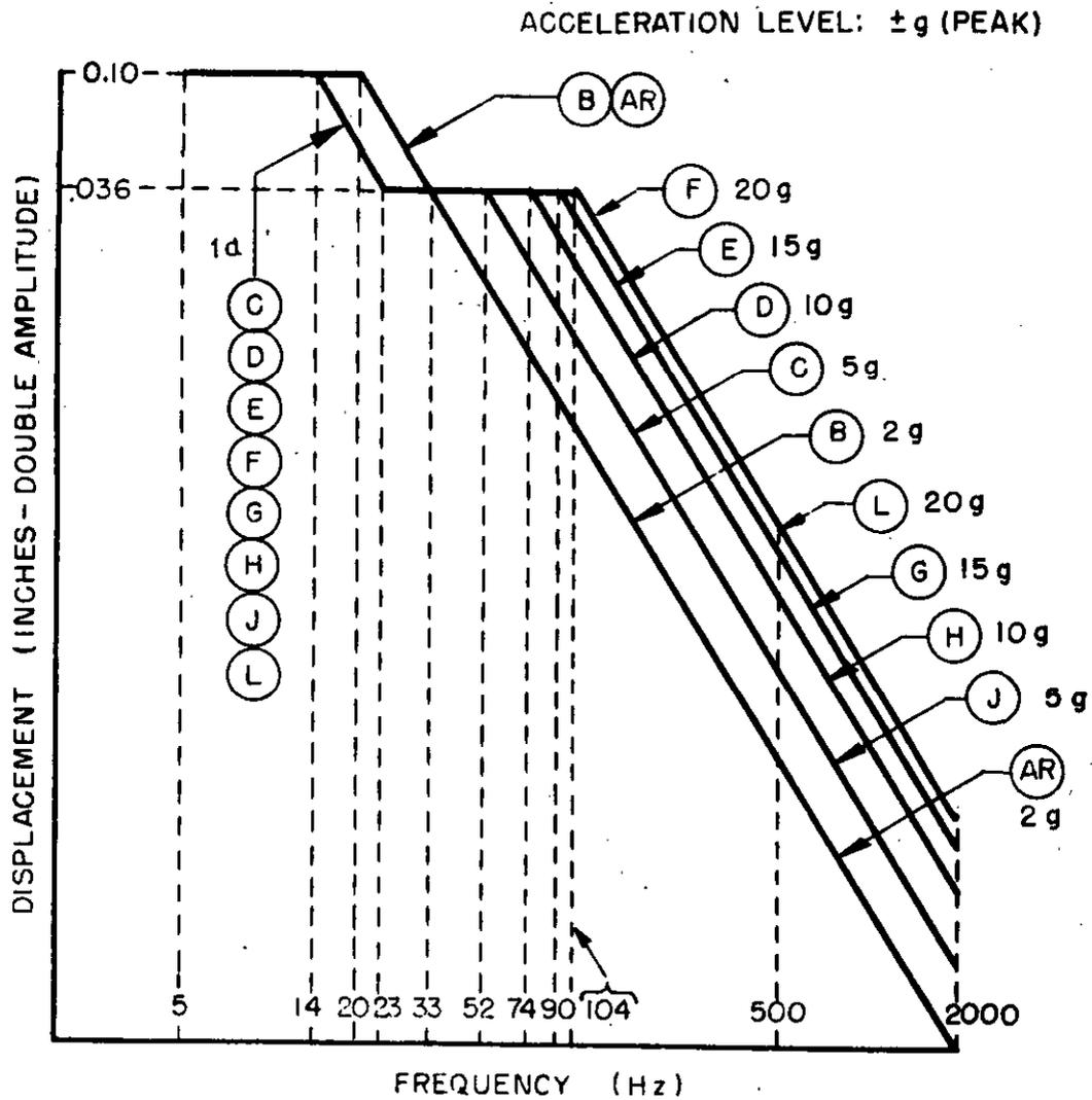
Figure 514.2-2. Vibration Test Curves for Equipment Installed in Airplanes, Excluding Helicopters, Equipment Category b.1.
