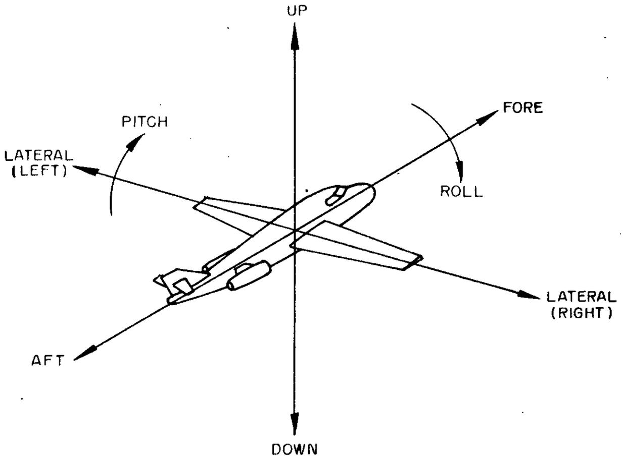
FIGURE 513.2-1. Direction of Vehicle Acceleration
