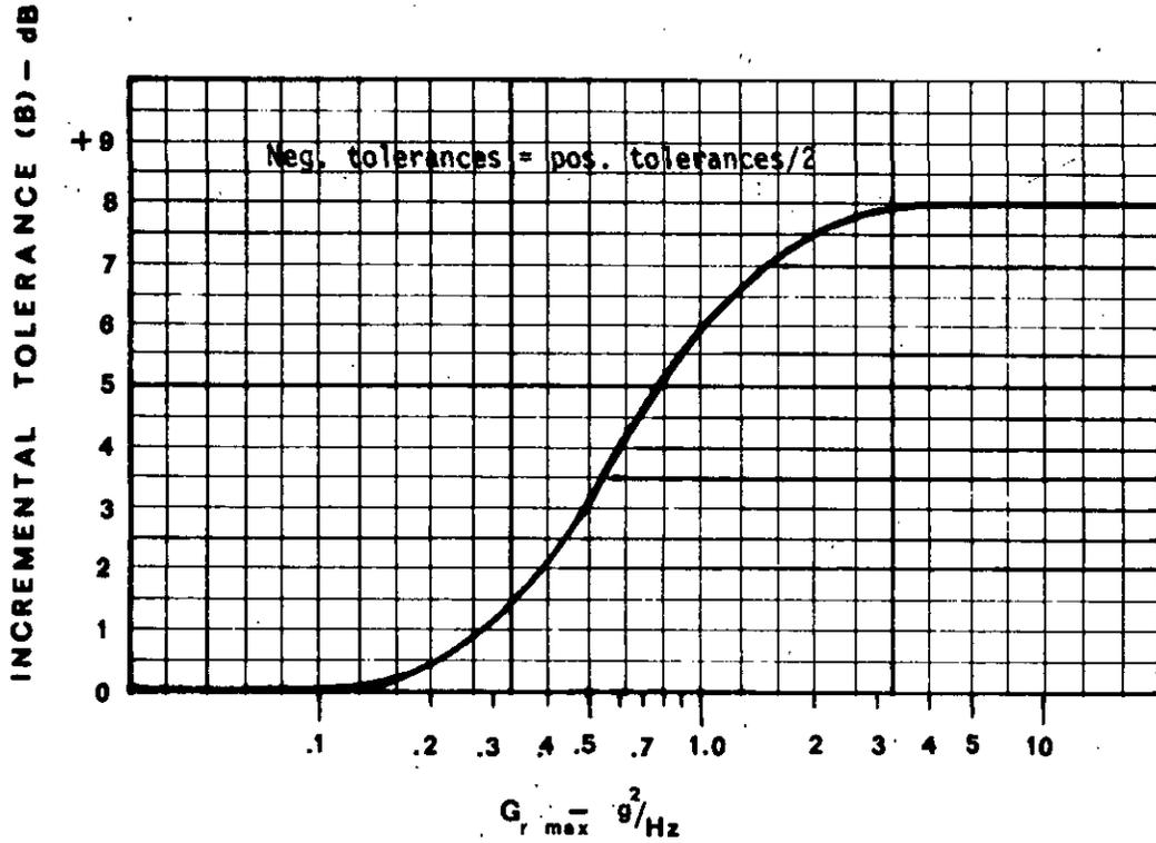
FIGURE 519.2-21 Gunfire test tolerance (B) for  $G_{r \max} \geq 0.1 g^2/Hz$
