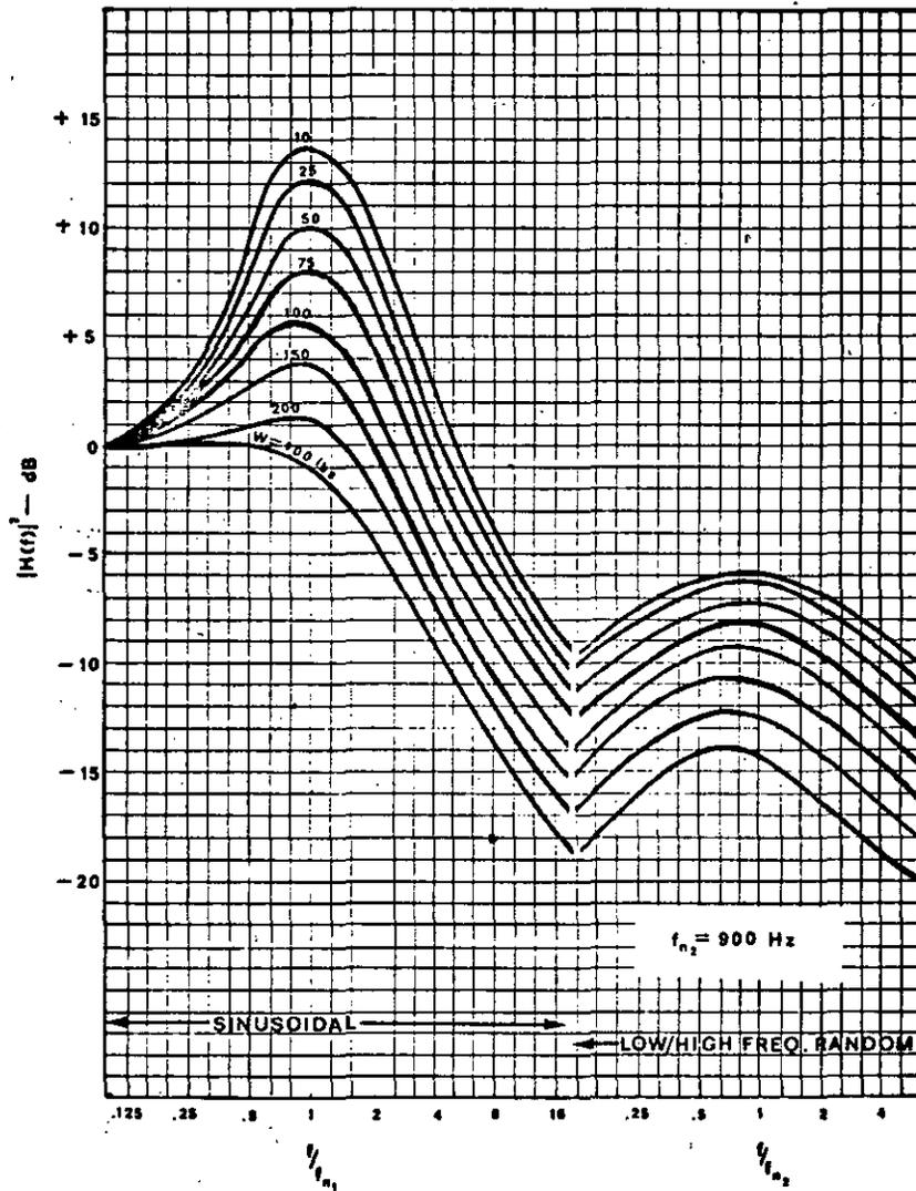
FIGURE 519.2-19 Transfer functions for non-isolated equipments
