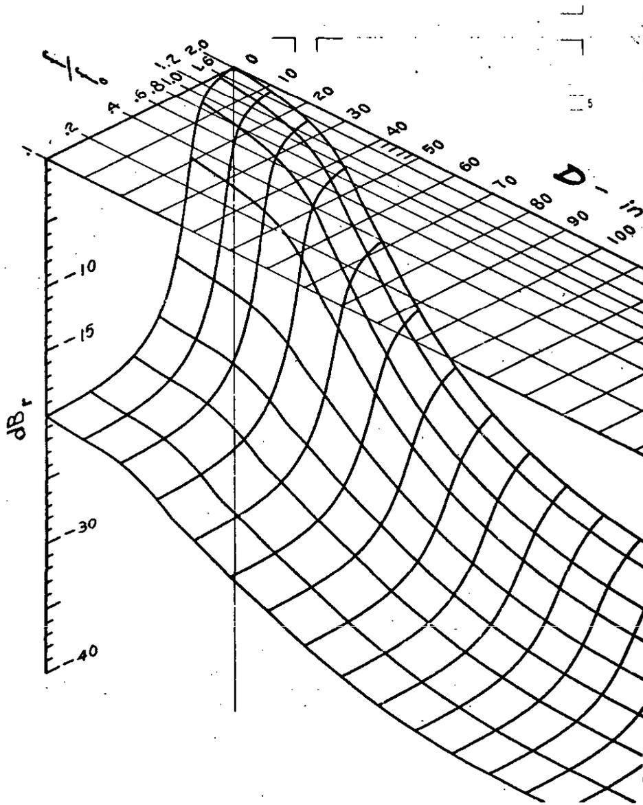
FIGURE 519.2-4. Random vibration prediction surface, low frequency
