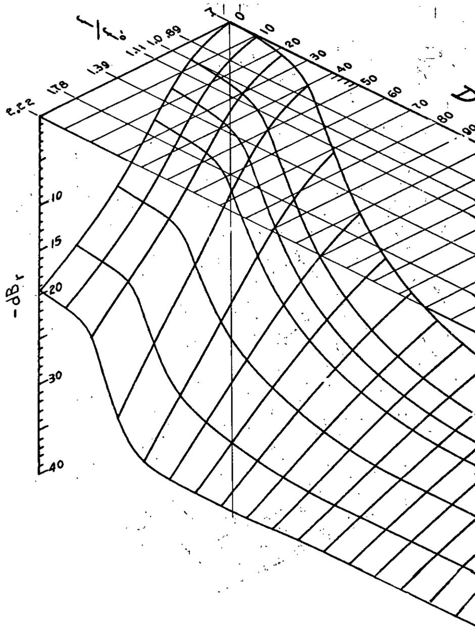
FIGURE 519.2-3. Random vibration prediction surface, high frequency
