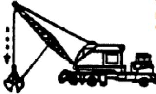
then release primary drum brake pedal to lower clamshell bucket over material.
