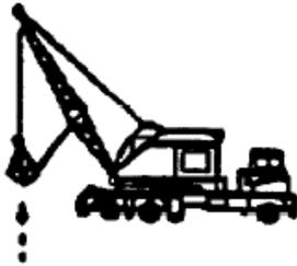
both levers back until the load has reached the desired height. Return both drum clutch levers to neutral and at the same time apply both drum brake pedals.
