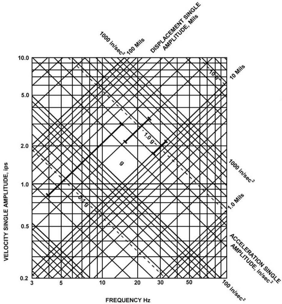
FIGURE 1. Type I environmental vibration limits (black bars represent a graphical presentation of table I expressed in displacement, velocity, and acceleration).
