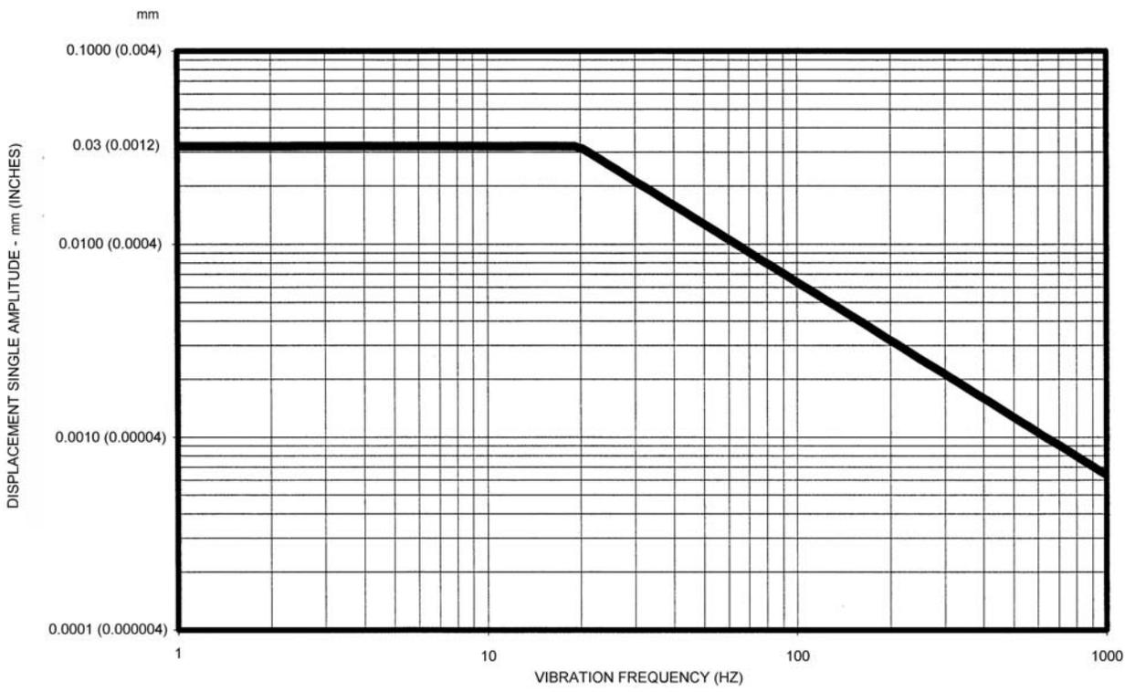
FIGURE 2. Vibration acceptance criteria for Type II vibration.
