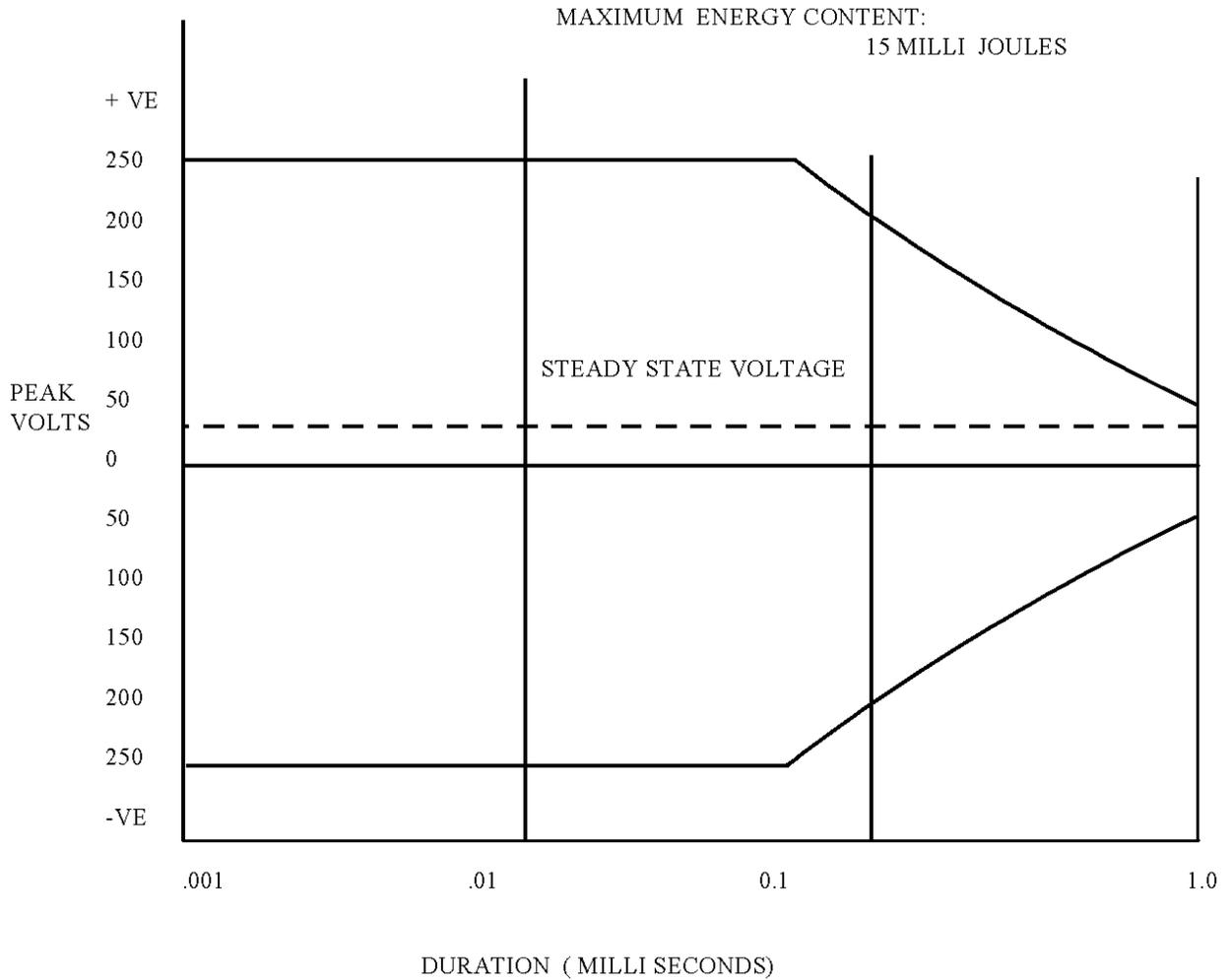
FIGURE A-3. Loci of spikes - fault free conition.
