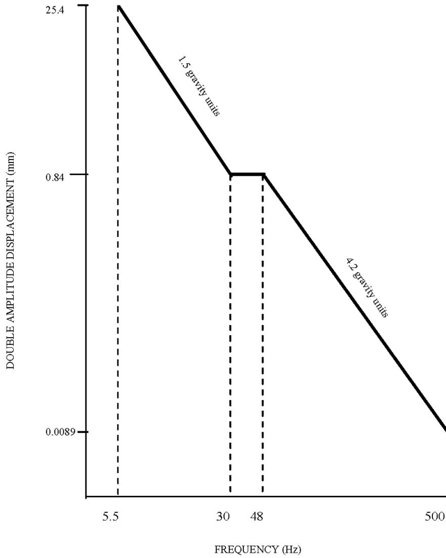
FIGURE 10. Vibration test curve.
