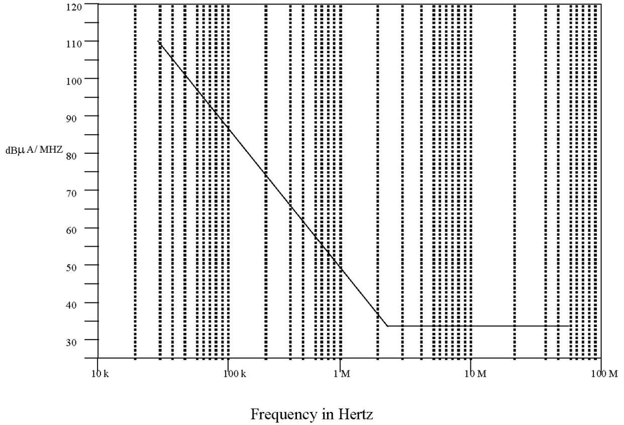
FIGURE 2. Conducted emissions (30 Hz – 50 kHz) - broadband emissions.
