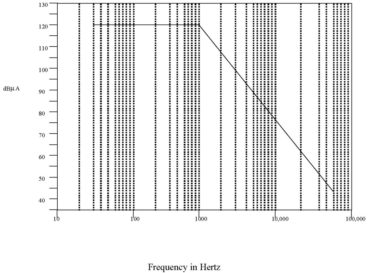
FIGURE 1. Conducted emissions (30 Hz to 50 kHz) - bandwidth limit.
