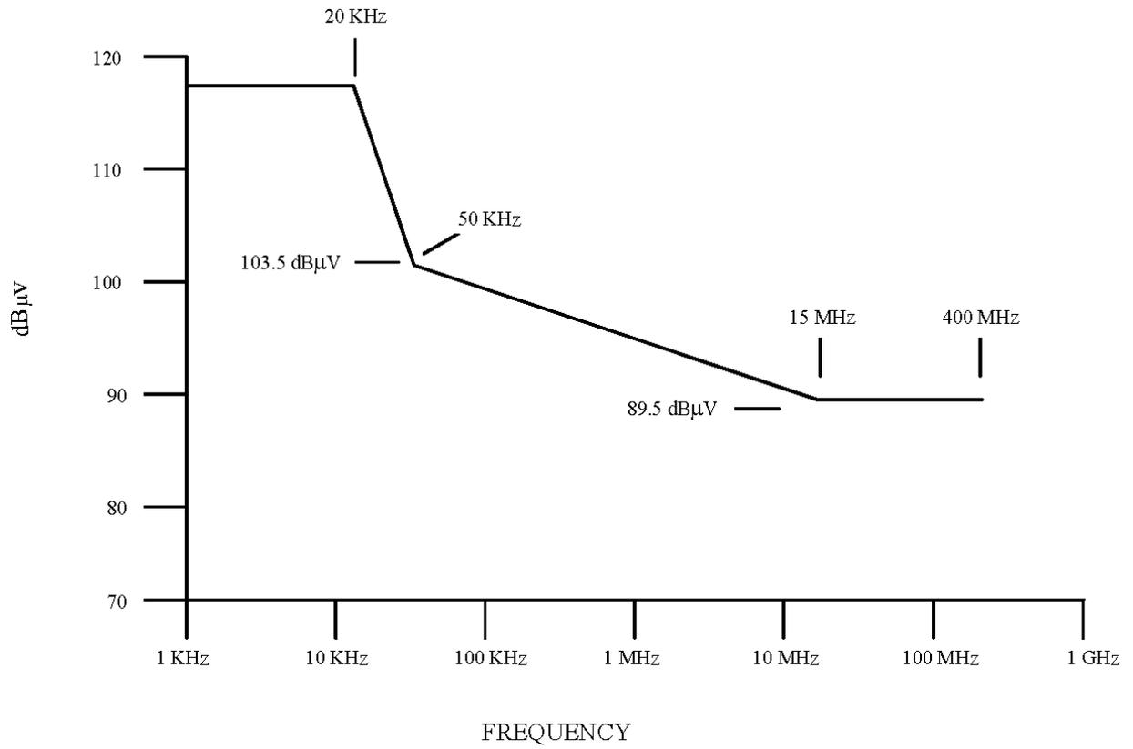
FIGURE 9. Radiated susceptibility - narrowband conducted emissions limit.
