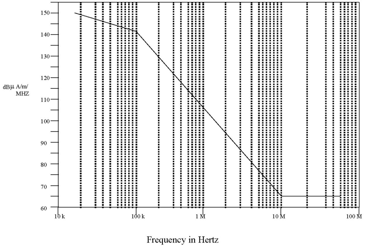
FIGURE 4. Conducted emissions (10 kHz to 50 MHz) - broadband emissions.
