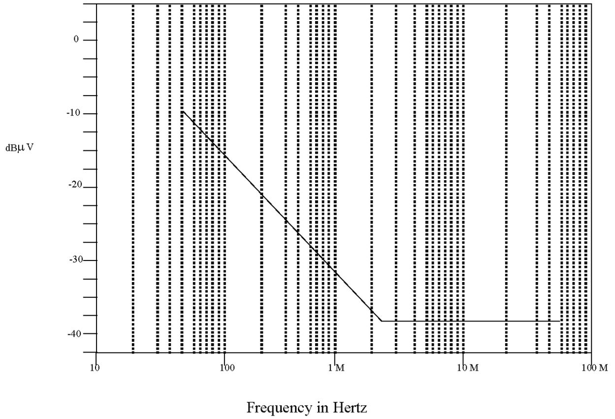
FIGURE 6. Conducted susceptibility (50 kHz to 400 MHz) - voltage limit.
