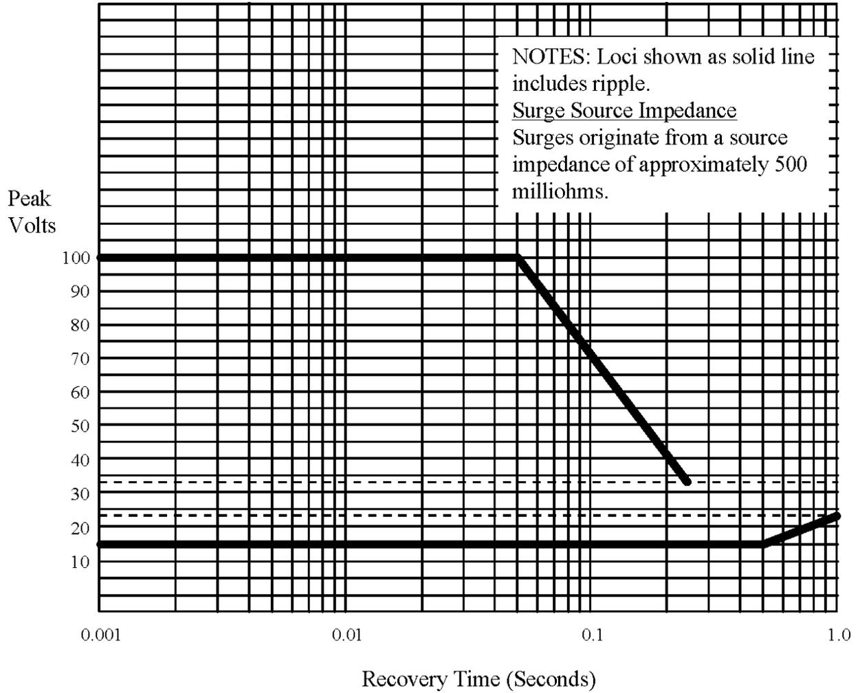
FIGURE A-4. Loci of surges - single fault condition.
