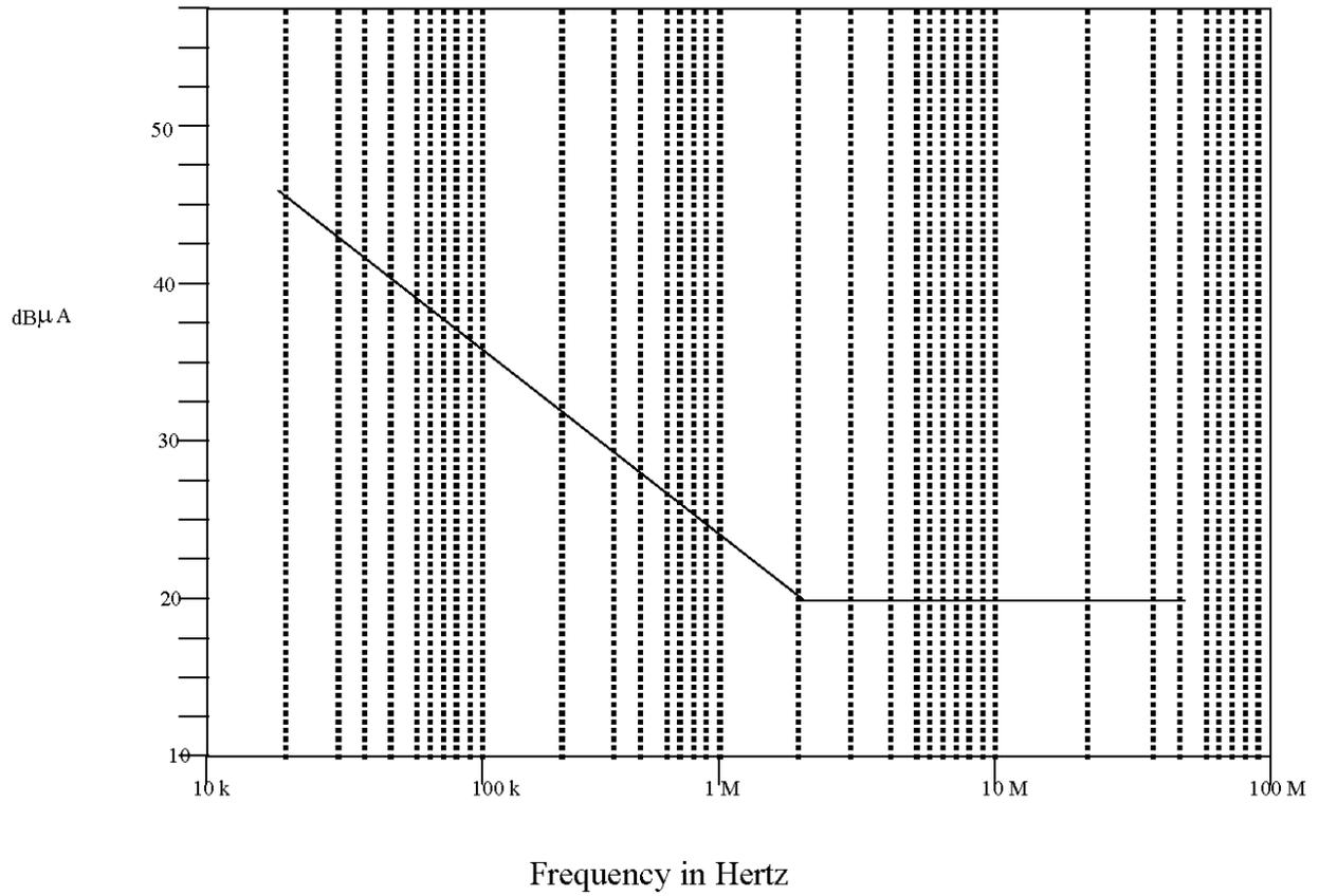
FIGURE 3. Conducted emissions (10 kHz to 50 MHz) - narrowband emissions.
