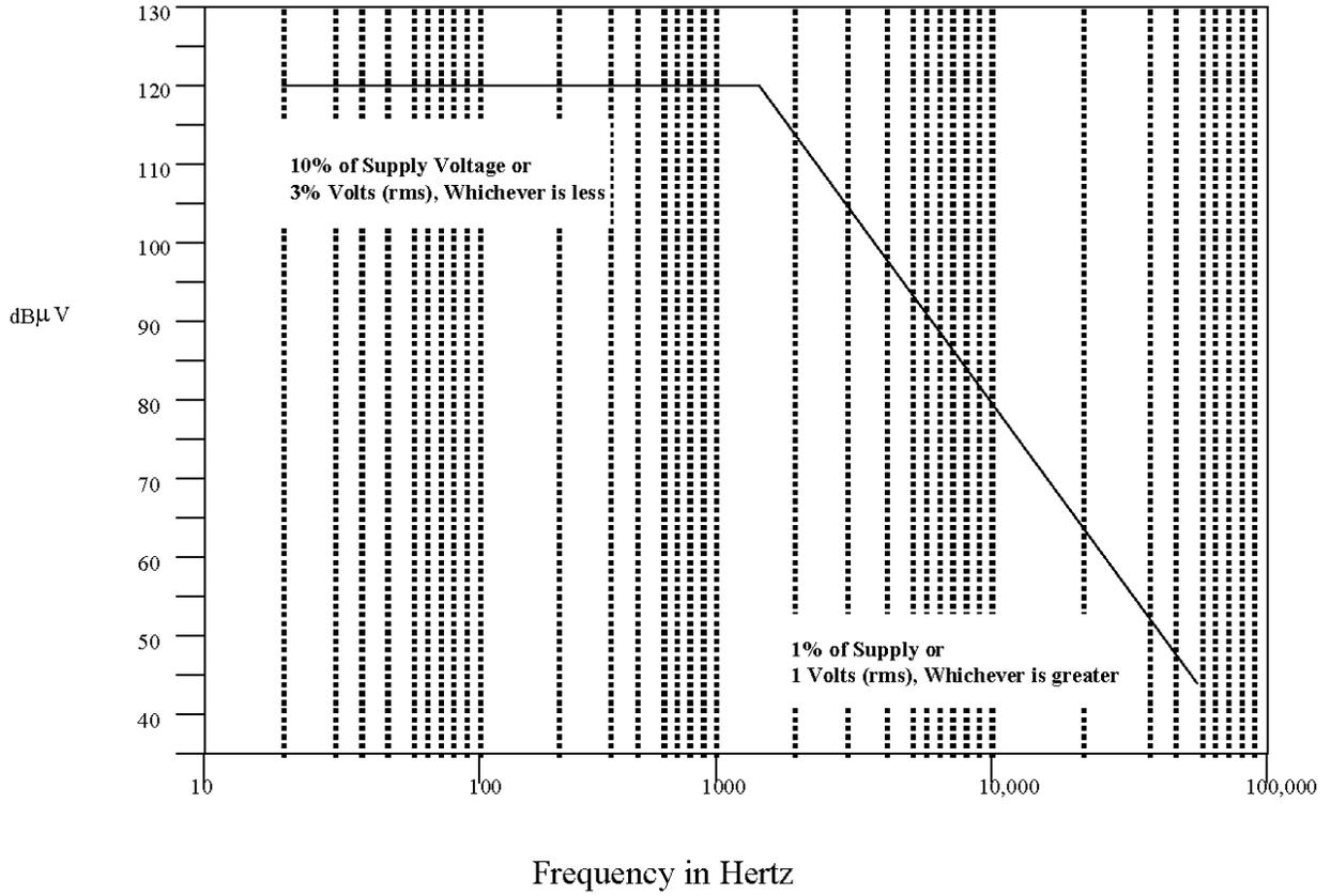
FIGURE 5. Conducted susceptibility (30 Hz to 50 KHz) - voltage limit.
