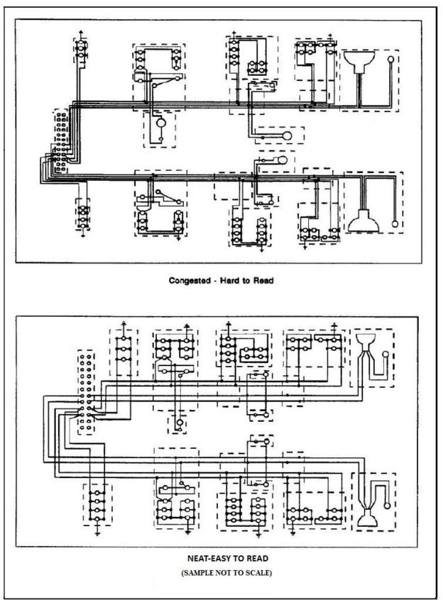
FIGURE 26. Example line separation on diagrams.
