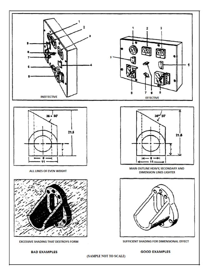
FIGURE 25. Examples of angle view, line weight, and shading.
