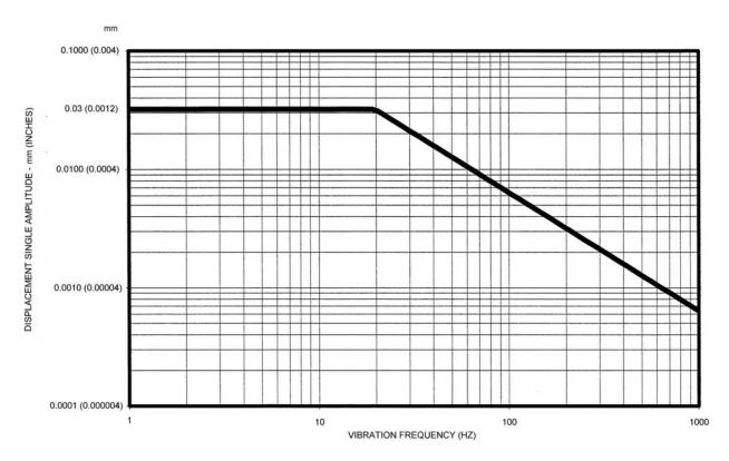
FIGURE 2. Vibration acceptance criteria for Type II vibration.
