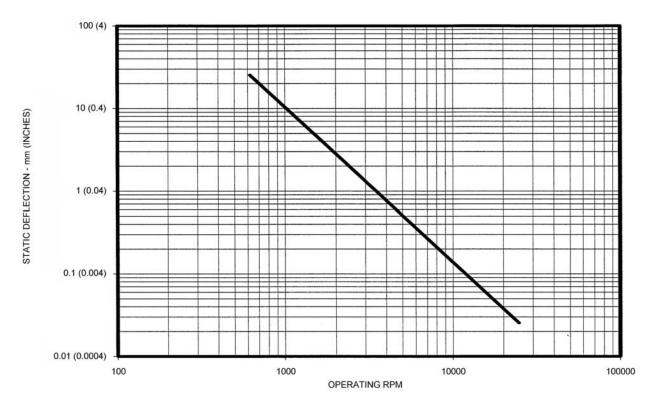
FIGURE 3. Minimum static deflection of mounting for Type II vibration test.
