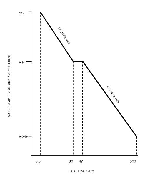
FIGURE 10. Vibration test curve.
