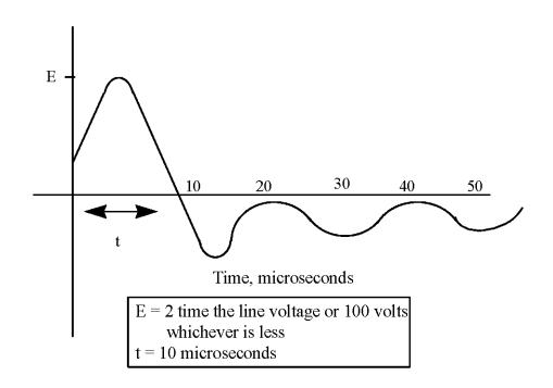
FIGURE 7. Spike - voltage limit.
