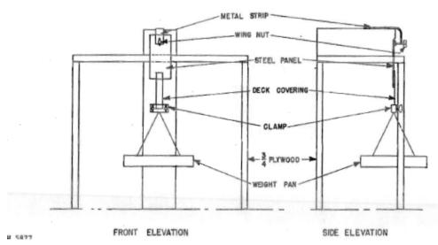
FIGURE 4. Adhesion testing machine.
