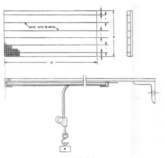
FIGURE 6. Strip adhesion test.
