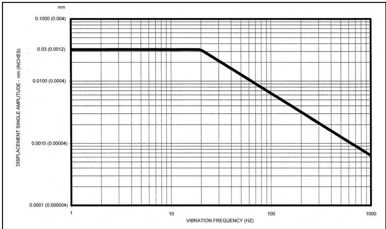
Figure 528-2. Vibration acceptance criteria for Type II vibration.
