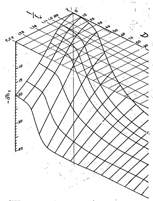
FIGURE 519.2-3. Random vibration prediction surface, high frequency
