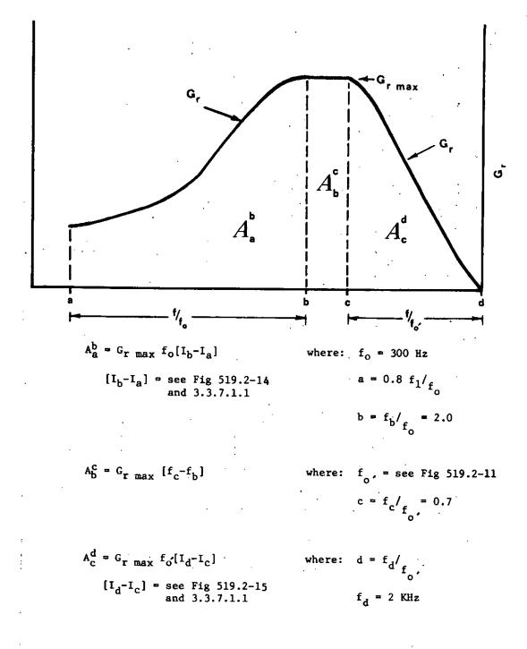
FIGURE 519.2-13. Determining the OAMS from the random test curves
