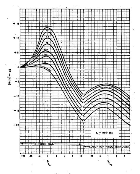
FIGURE 519.2-19 Transfer functions for non-isolated equipments
