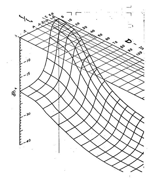
FIGURE 519.2-4. Random vibration prediction surface, low frequency
