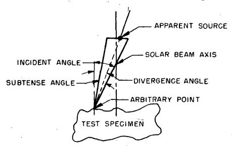
Figure 517.2-1. Geometrical Relationship of Solar Subtense and Incident Angle
