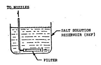
Figure 509.1-3 Location of Salt Solution Filter
