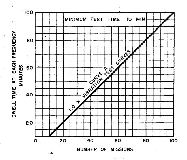
Figure 514.2-4C. Time Curves for Dwell Test for Externally Carried Stores for Helicopters, Equipment Category d.3.
