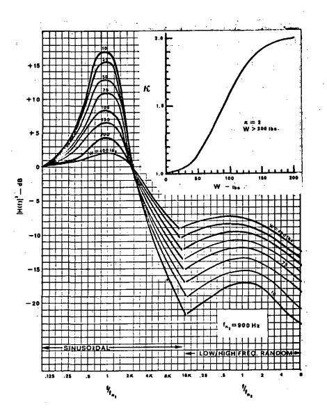
FIGURE 519.2-18 Transfer function for isolated equipments
