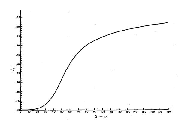
FIGURE 519.2-16. Slope factor,  $\beta_{f},$  for the low frequency random surface
