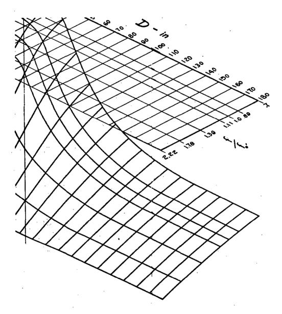
FIGURE 519.2-3. Random vibration prediction surface, high frequency (Cont'd)
