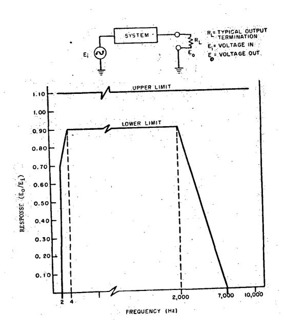
FIGURE 516.2-3. Shock Measuring System Frequency Response
