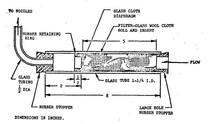
Figure 509.1-2 Salt Solution Filter
