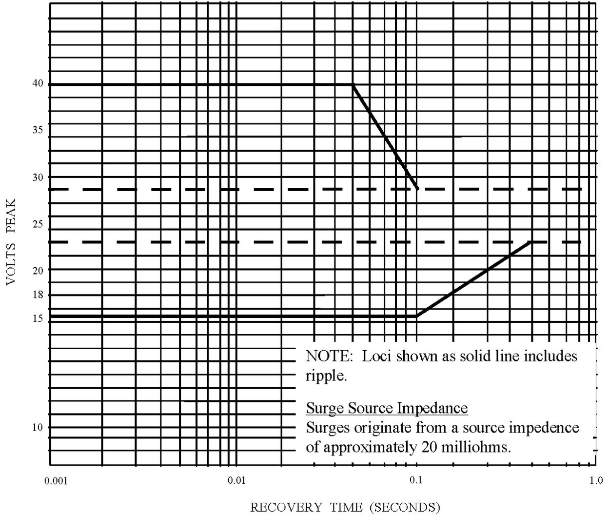
FIGURE A-2. Loci of surges - fault free condition.
