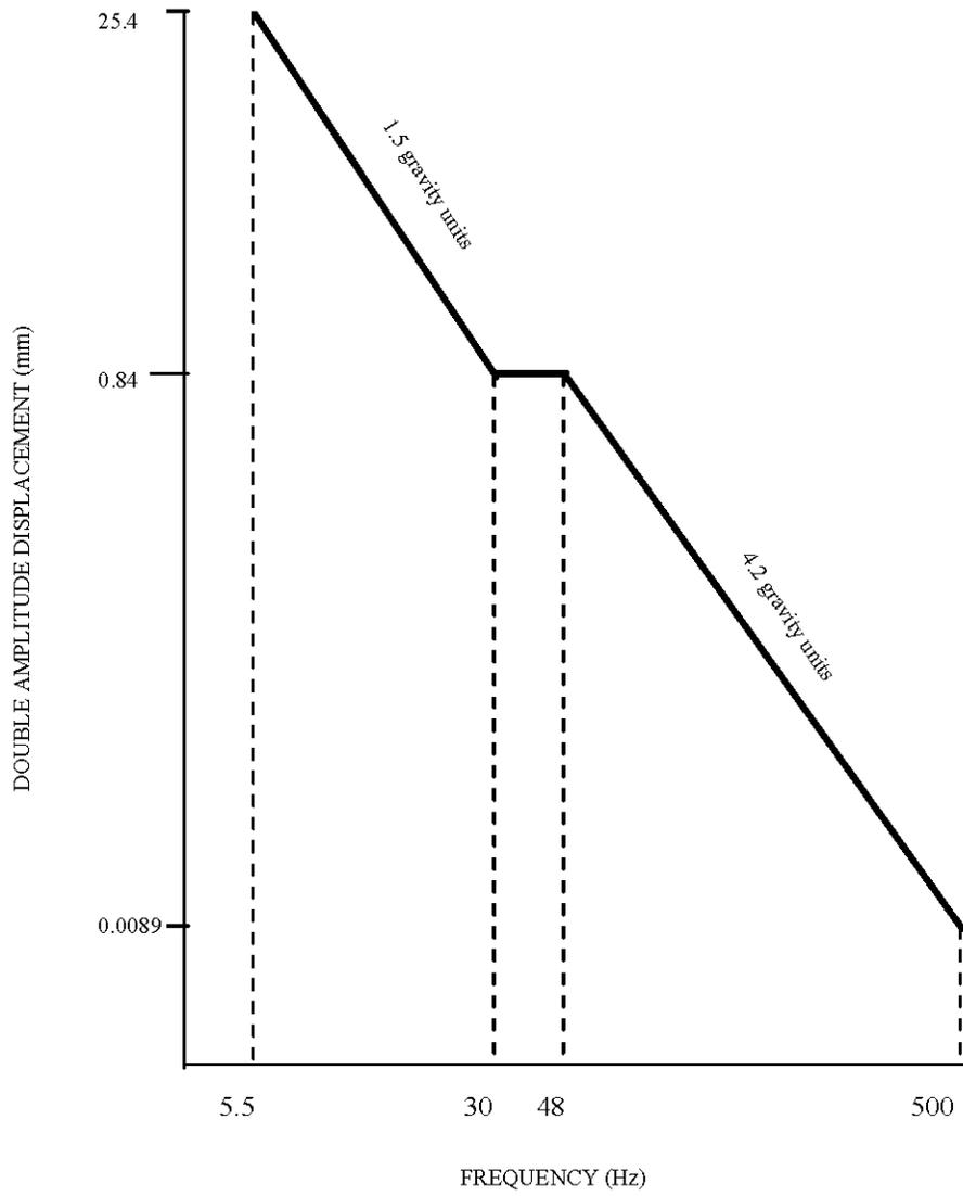
FIGURE 10. Vibration test curve.
